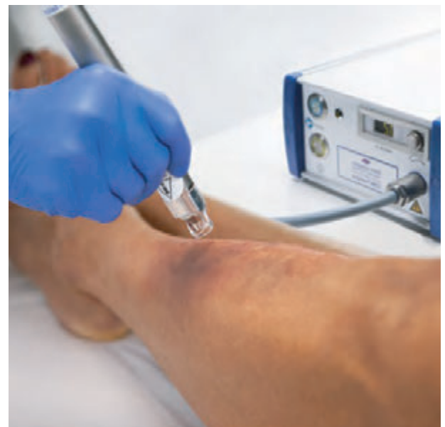
KINPen® MED: This CE-certified atmospheric plasma jet for medical applications is produced by neoplas med GmbH
